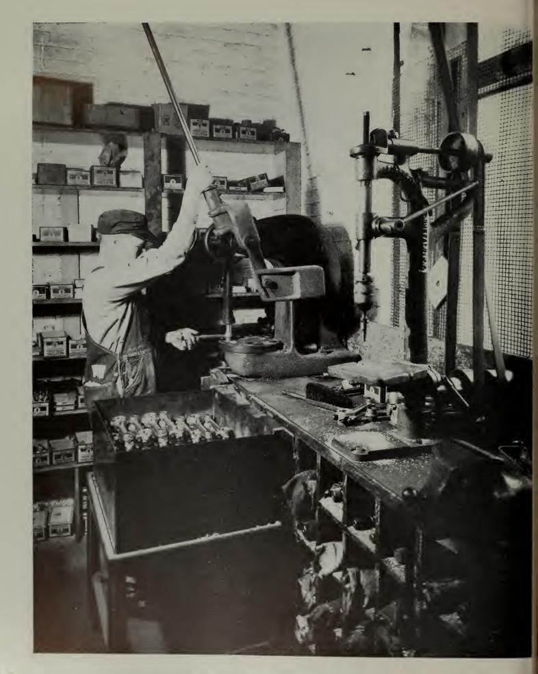
About one half of the connecting rods rebabbitted require new bushings in small end of the shank. These are installed by a hand operated arbor press, as shown above.
